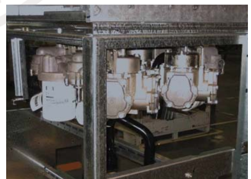
Encore with T19976-G5 Flex Fuel Meter
